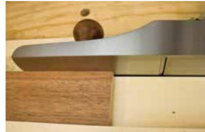
When starting out there will be a gap between the shooting board and the plane. The smaller the gap gets, the closer you are to being finished
