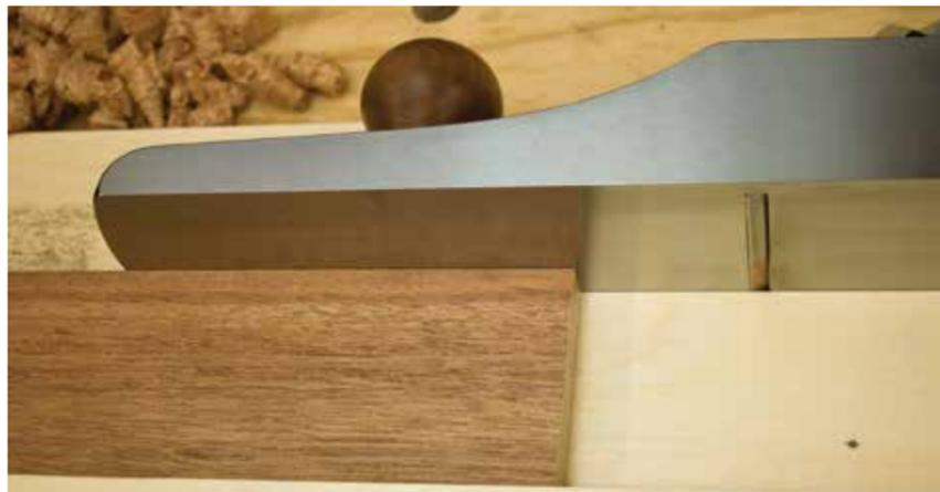
When the plane bottoms out on the shooting board and stops cutting, you're done
