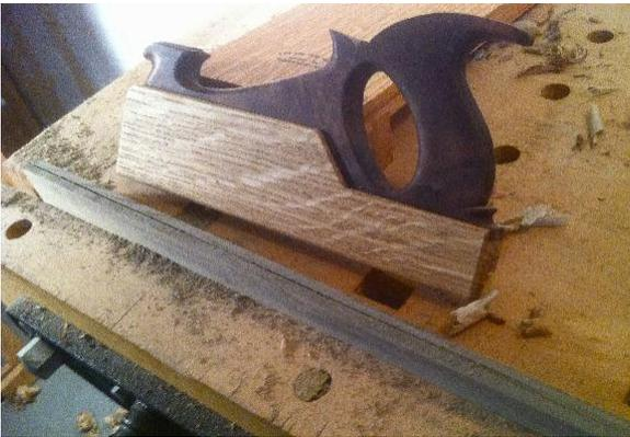
This kerfing saw, made by Tom Fidgen, pre-kerfs a board’s edge a set distance from the board’s face. He then uses a hand saw to rip the board from end to end, re-sawing the wood. The pre-kerf tracks the saw along the cut.
