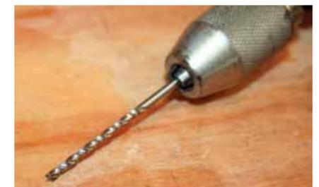
Unless you're a collector, you shouldn't feel compelled to track down the original straight-fluted bits – modern bradpoint bits work better and are readily available
