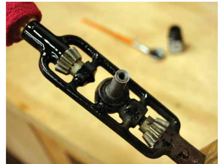
Wrap the handle in a cloth or cling film to keep it clean then start painting the body. Take your time and keep the paint clear of the gears and oil holes. I like to clamp the chuck post in a rubber-jawed vice so I can rotate the drill as I work and then walk away to let it dry
