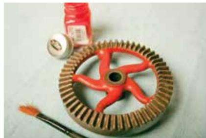
Painting the main gear is simple, just try to avoid getting paint between the gear teeth
