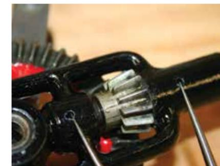
There are typically two or more oil holes as shown here. Clean the holes out with a nail if need be, then add some lightweight machine oil and work it into the gears
