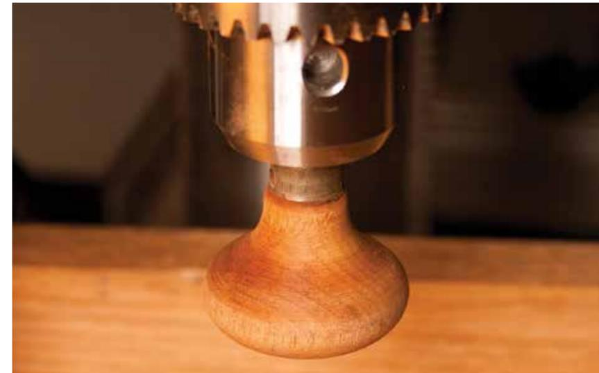
Chuck the side knob into the drill press and start sanding
