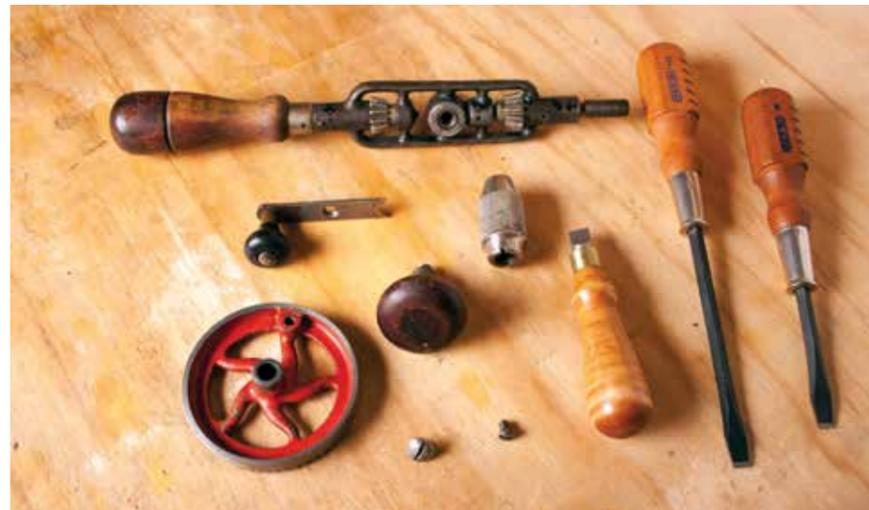
Using properly sized screwdrivers, disassemble the drill as shown
