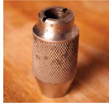
Leave the chuck assembled unless it absolutely requires a full cleaning. You can see the slots on the top of the chuck where a tool can unscrew the top from the body. The top portion of the chuck stops right where the knurling pattern begins
