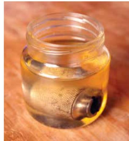
Drop the chuck in some penetrating oil, like WD-40, and let it soak for several hours to loosen up jaws and springs
