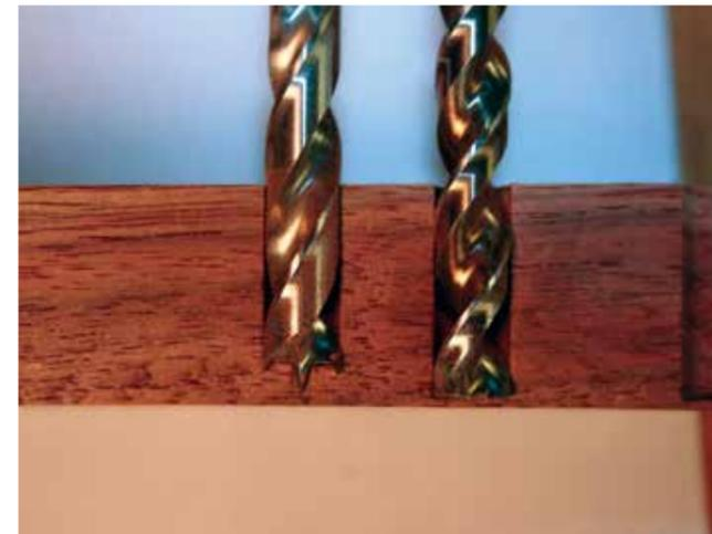
A comparison of two holes shows the advantage of drilling a second time with a flat bit. Now the magnet can sneak right up to the front face
