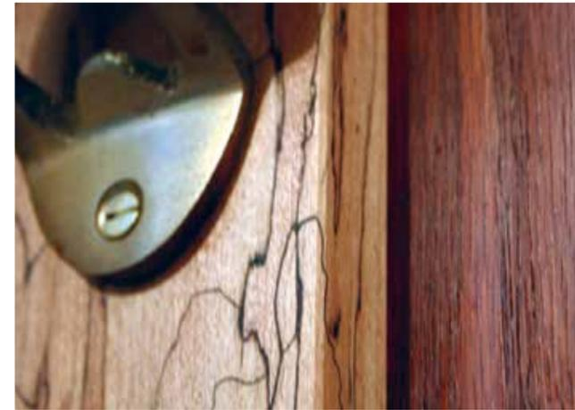
Note the continuous grain lines running from the face through the edges of the board, made possible using the 'plug method'
