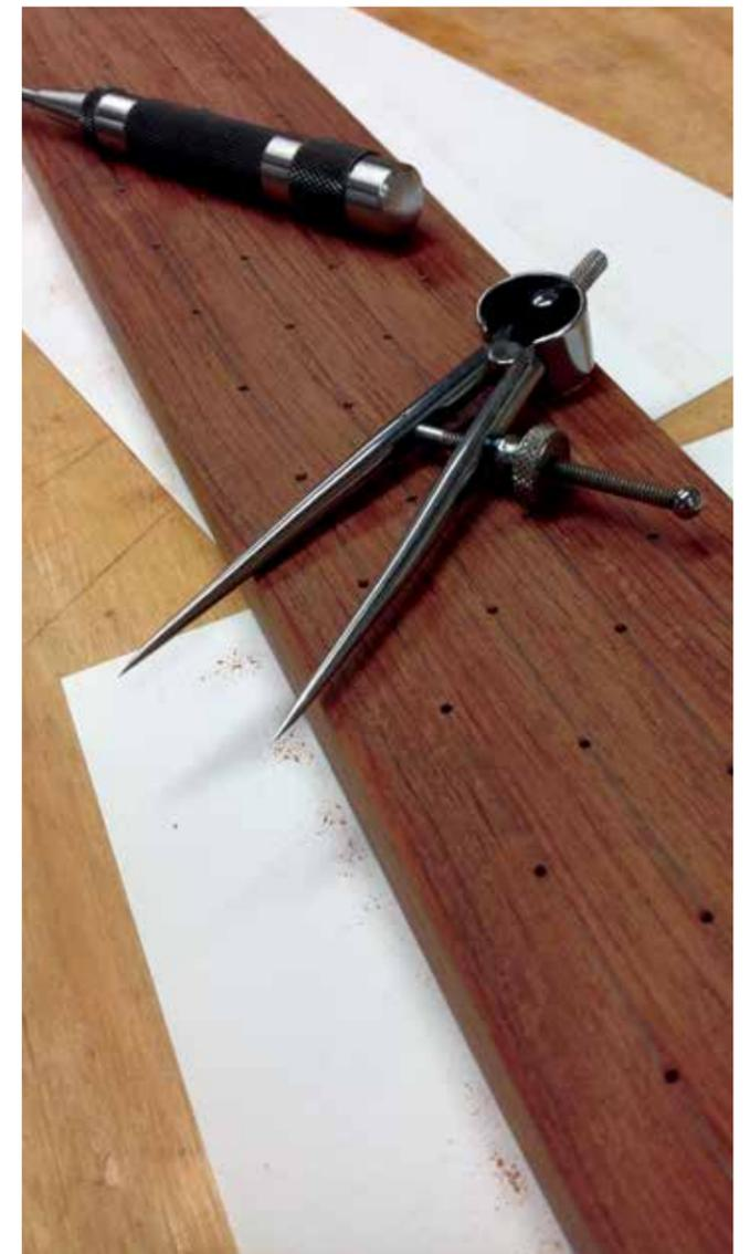
Lay out the pattern for your magnets - dividers help - then get to drilling
