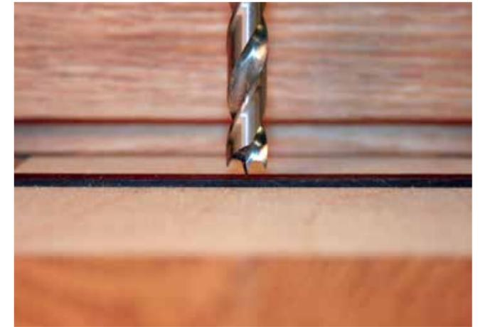
Install a sharp bit and set the depth stop on your drill press to stop the bit when the tip just touches a 0.5mm shim
