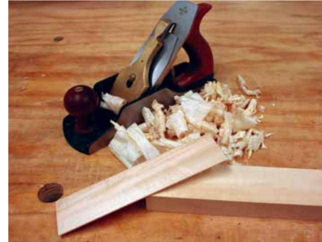
After resawing, remove the saw marks to leave a clean, flat surface for installing the magnets and reattaching the face
