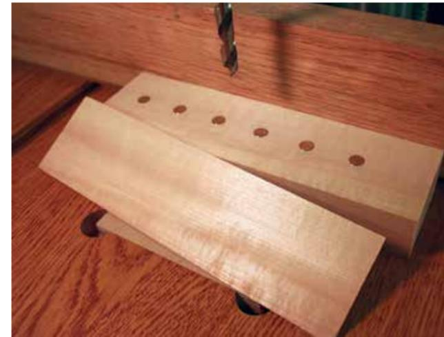
Drill the holes just deep enough for the magnets to sit flush in the body, then glue the face back on
