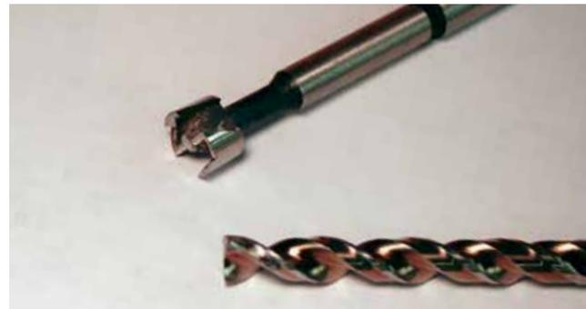
Twist bits or Forstner bits can be ground flat for cleaning out the bottom of holes
