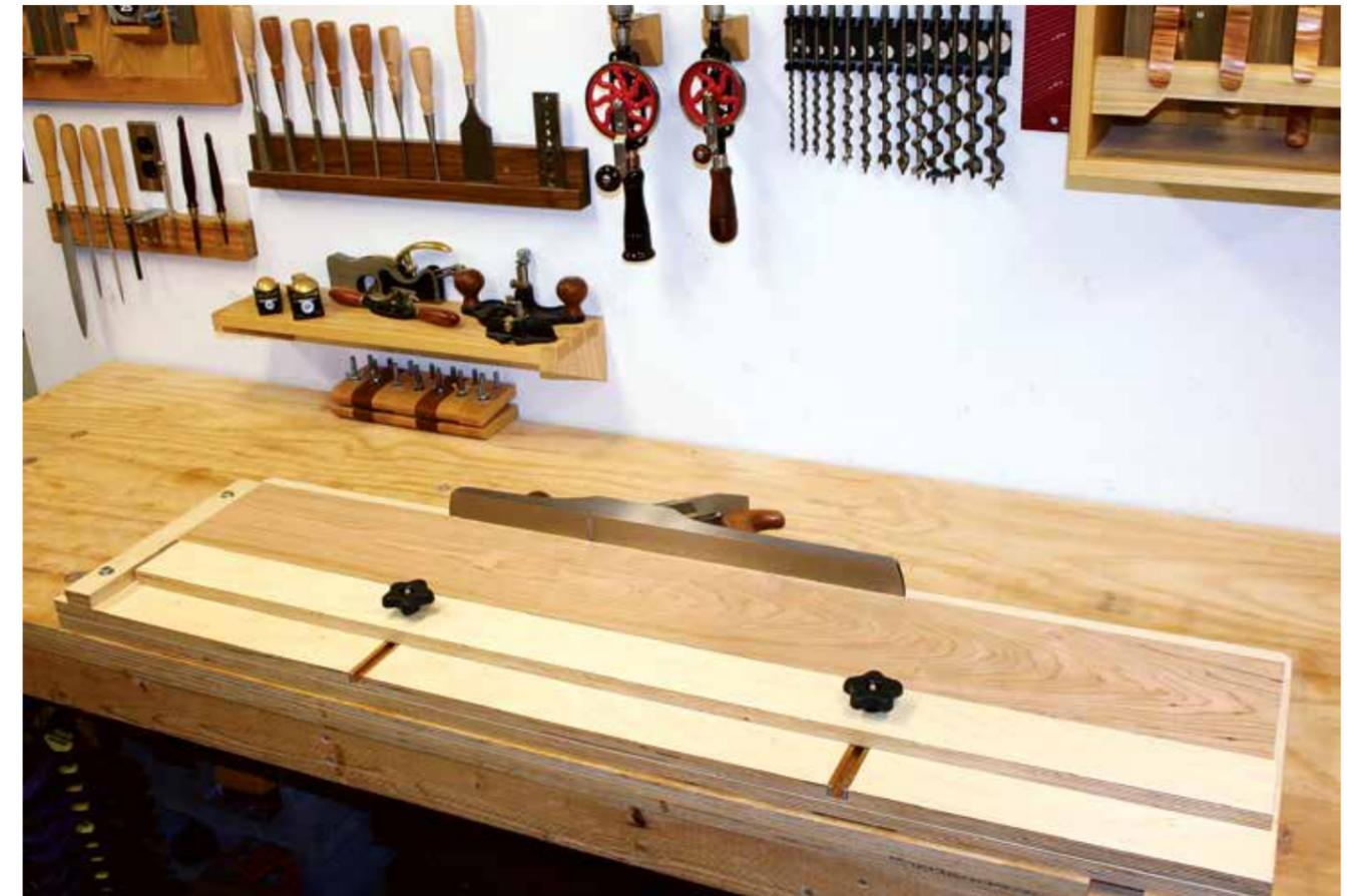
Long grain shooting board with adjustable fence for repeatable board widths or tapers
