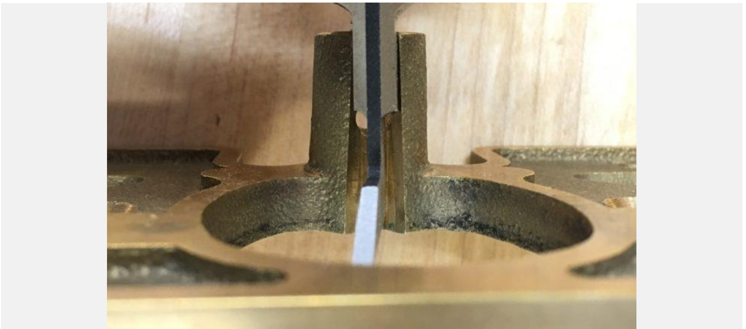
This is roughly the starting point for the blade where a flush cut would be taken. Notice how there isn't a lot of supporting material on the shank to align the cutter in the V-groove.
