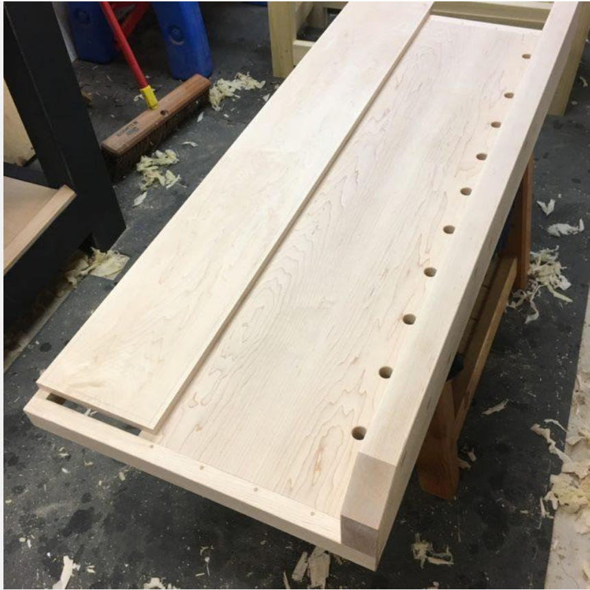
Laying out the bottom panel. You can also see the location of the breadboard pegs running through the underside of the bench.
