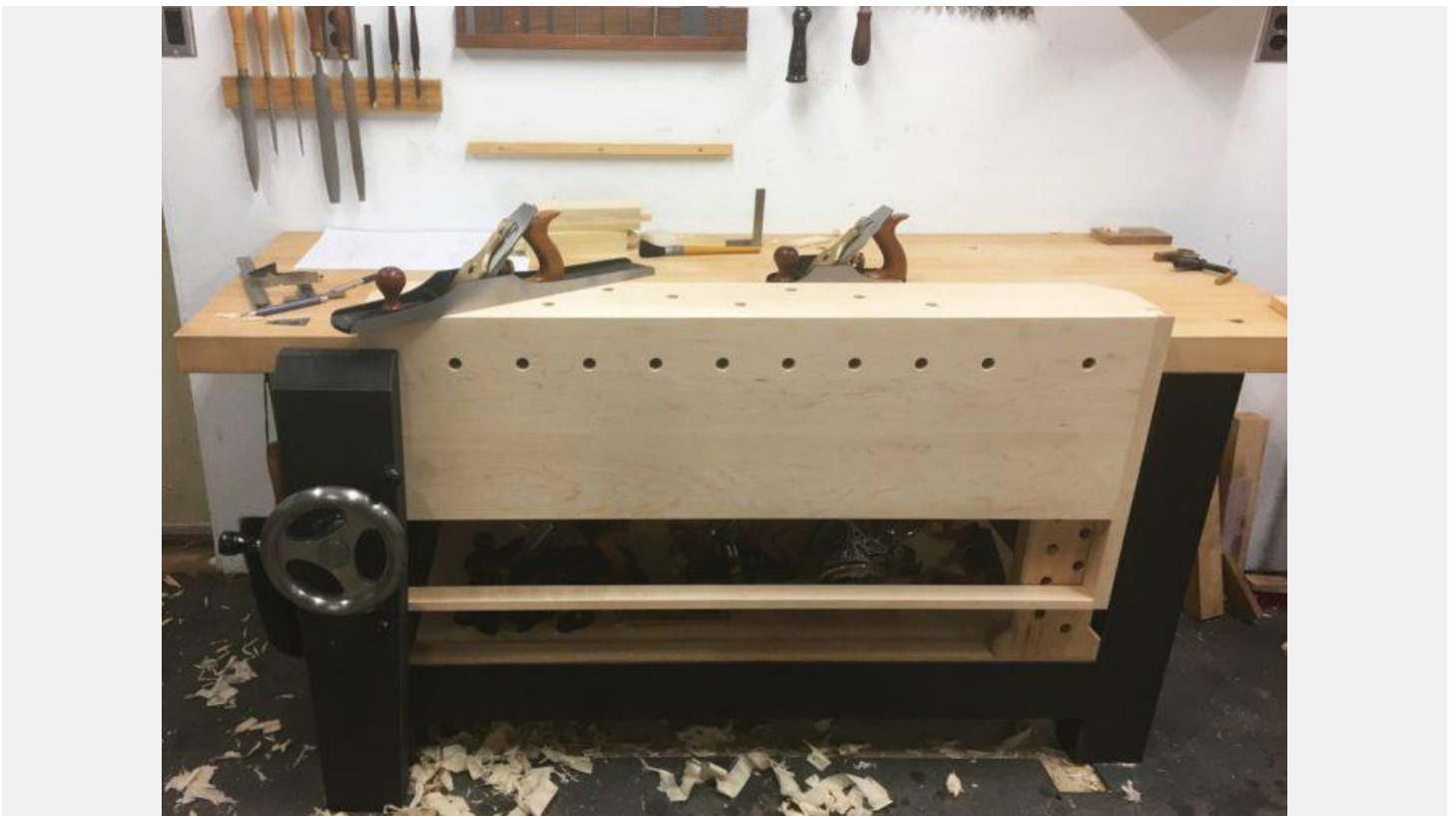
After the glue dries, make sure the apron is flat and square to the bench top surface.
