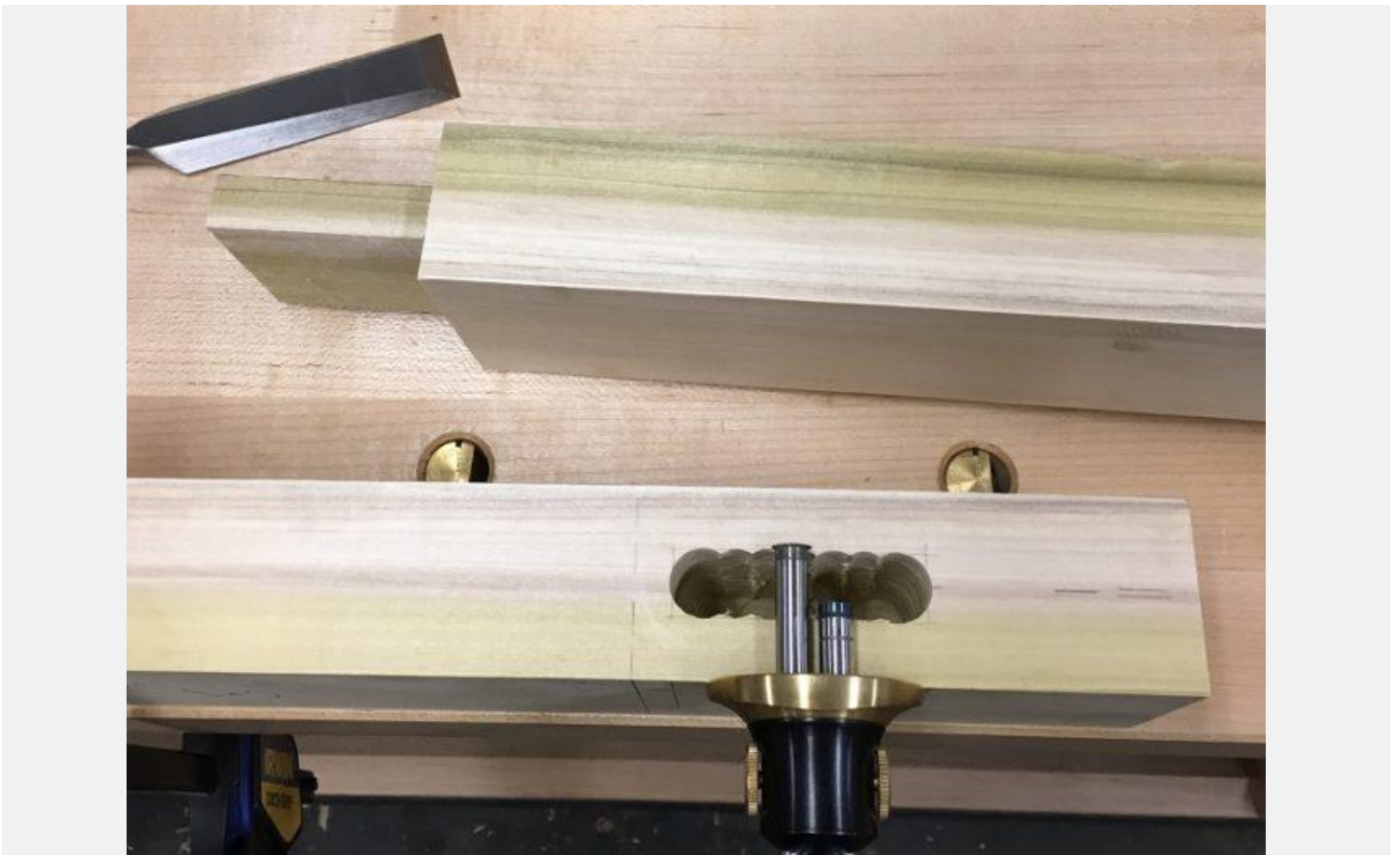
Lay out the mortises referencing off the same face. Use 2 different gauges or a dual mortise gauge like this one from Veritas.
