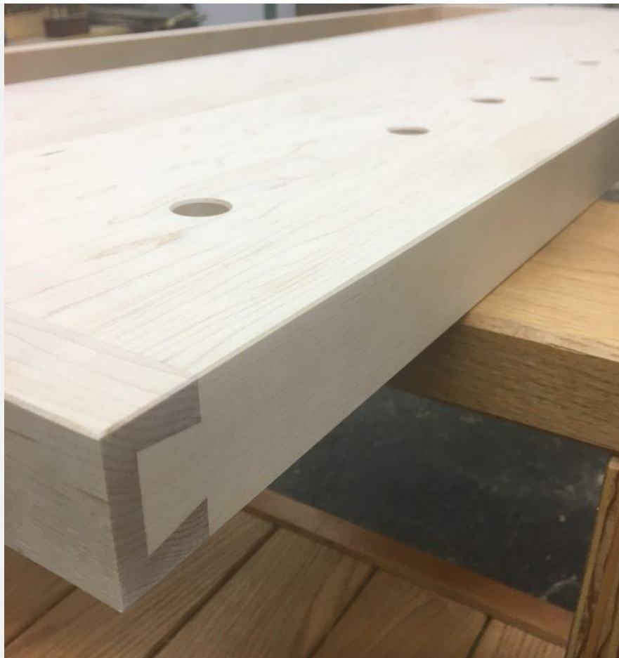
Completed breadboard end rail with dovetail key.
