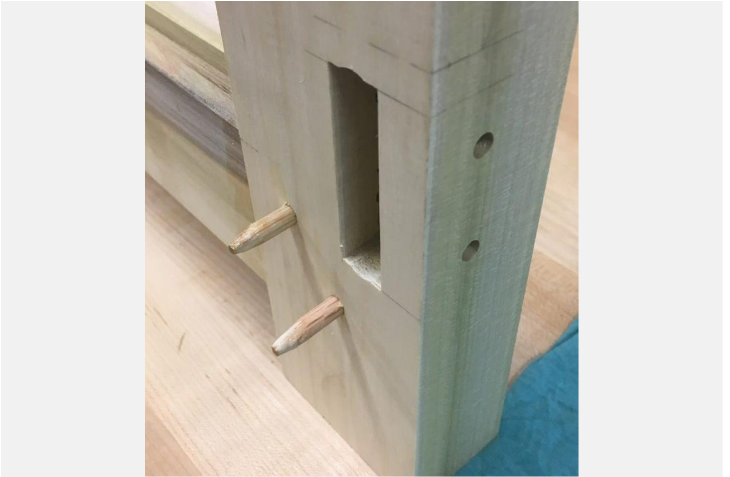
After the pegs are driven home they will get cut off on each side with a flush cut saw. Notice the pointed tips of the peg.
